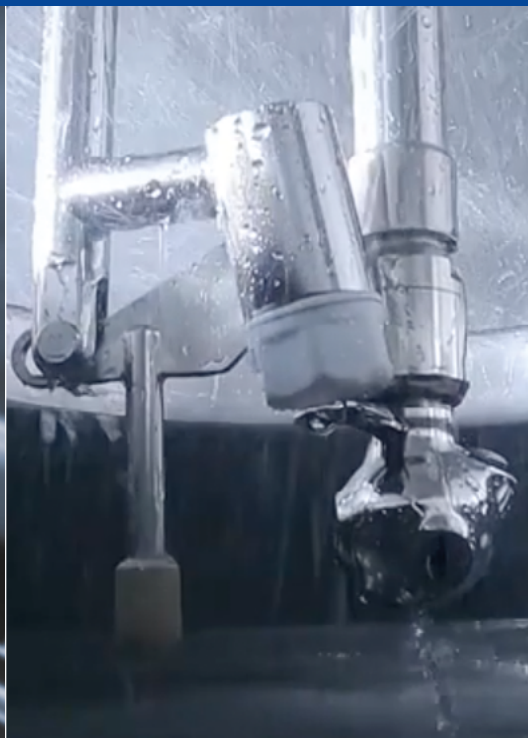
Internal cleaning via rotation-monitored high-performance spray head > Watch video on youtube.com
